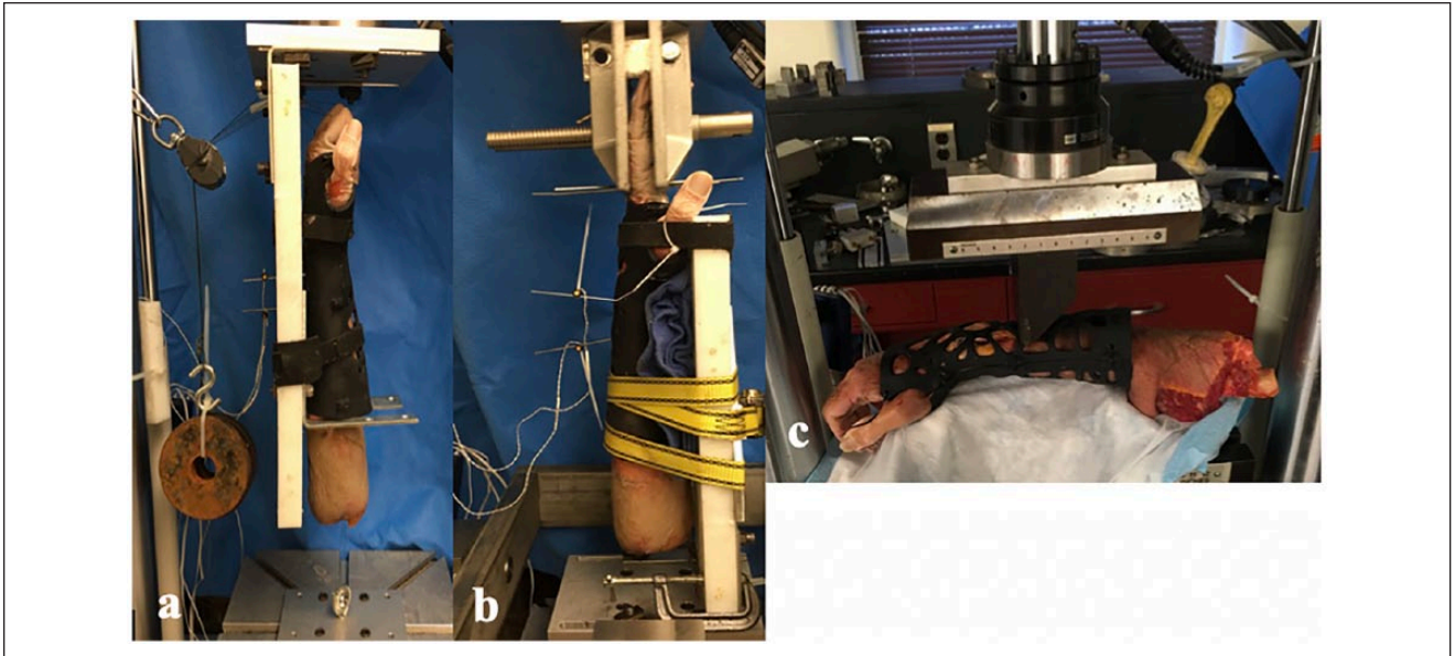
Figure 2. Mechanical testing setup: (a) flexion-extension, (b) pronation-supination, and (c) 3-point bending.
